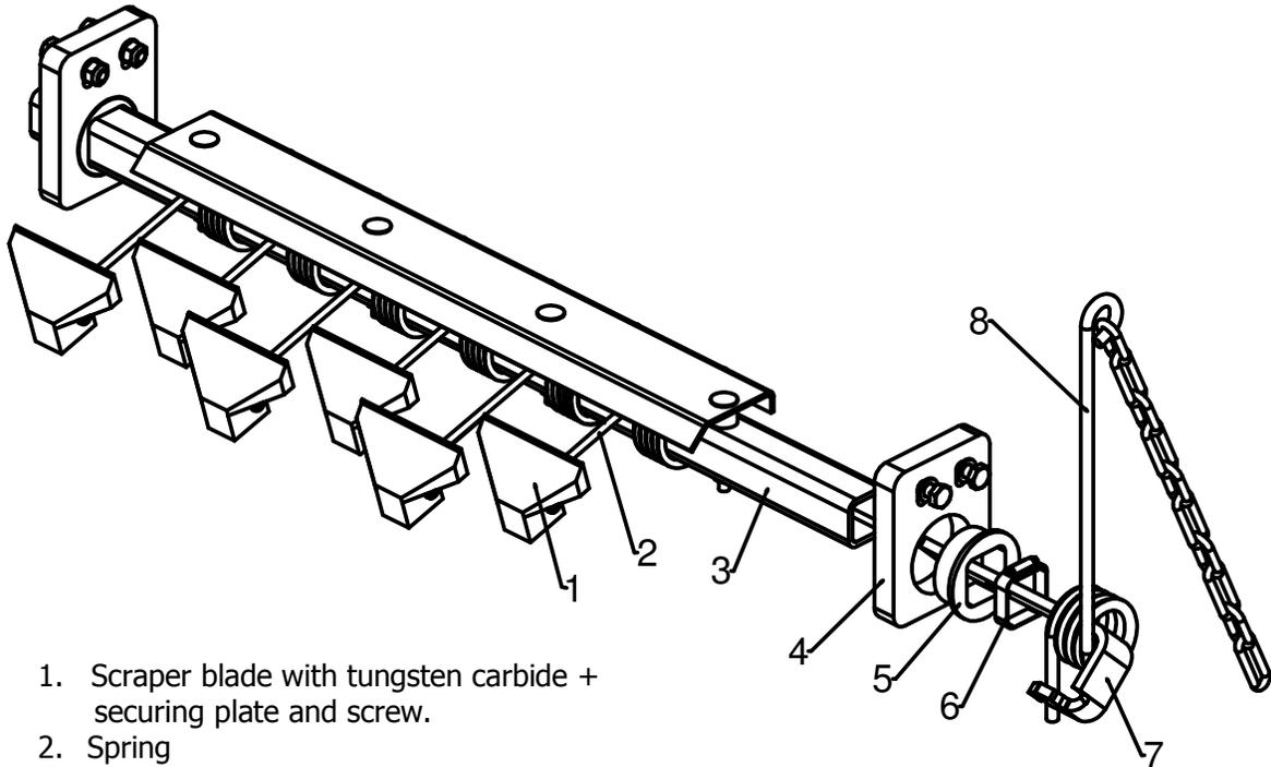
1. Scraper blade with tungsten carbide + securing plate and screw.
